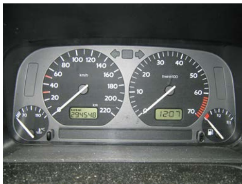
Figure 21.29 The fuel and temperature gauges (far right and far left, respectively) in this 1996 Volkswagen are voltmeters that register the voltage output of “sender” units, which are hopefully proportional to the amount of gasoline in the tank and the engine temperature. (credit: Christian Giersing)
