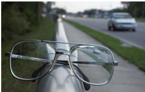
Figure 25.37 A car viewed through a concave or diverging lens looks upright. This is a case 3 image. (credit: Daniel Oines, Flickr)
