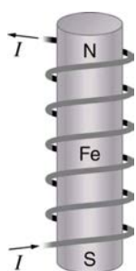
Figure 22.12 An electromagnet with a ferromagnetic core can produce very strong magnetic effects. Alignment of domains in the core produces a magnet, the poles of which are aligned with the electromagnet.
