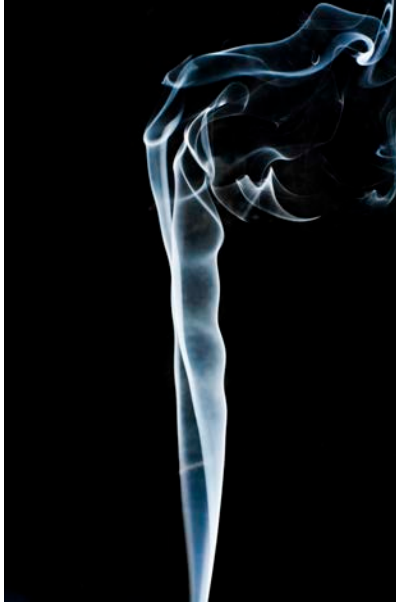
Figure 12.11 Smoke rises smoothly for a while and then begins to form swirls and eddies. The smooth flow is called laminar flow, whereas the swirls and eddies typify turbulent flow. If you watch the smoke (being careful not to breathe on it), you will notice that it rises more rapidly when flowing smoothly than after it becomes turbulent, implying that turbulence poses more resistance to flow. (credit: Creativity103)
