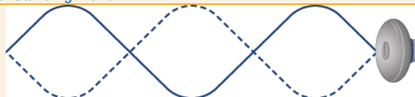
Figure 17.24 The standing wave pattern of a rubber tube attached to a doorknob.
