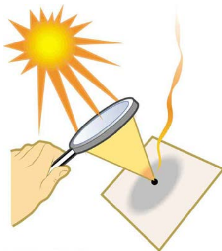
Figure 25.27 Sunlight focused by a converging magnifying glass can burn paper. Light rays from the sun are nearly parallel and cross at the focal point of the lens. The more powerful the lens, the closer to the lens the rays will cross.
