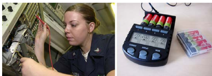
Figure 21.15 These two battery testers measure terminal voltage under a load to determine the condition of a battery. The large device is being used by a U.S. Navy electronics technician to test large batteries aboard the aircraft carrier USS Nimitz and has a small resistance that can dissipate large amounts of power. (credit: U.S. Navy photo by Photographer's Mate Airman Jason A. Johnston) The small device is used on small batteries and has a digital display to indicate the acceptability of their terminal voltage. (credit: Keith Williamson)
