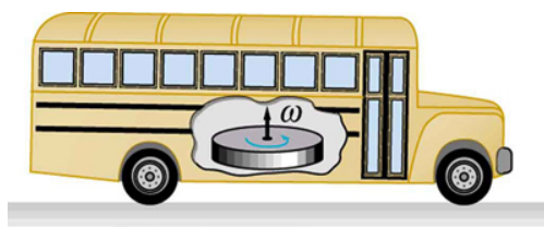
Figure 10.16 Experimental vehicles, such as this bus, have been constructed in which rotational kinetic energy is stored in a large flywheel. When the bus goes down a hill, its transmission converts its gravitational potential energy into KE_{\text{rot}} . It can also convert translational kinetic energy, when the bus stops, into KE_{\text{rot}} . The flywheel's energy can then be used to accelerate, to go up another hill, or to keep the bus from going against friction.
