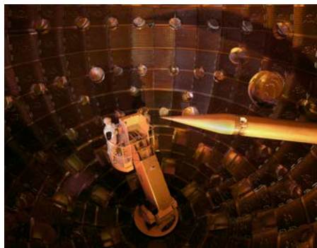
Figure 30.41 This system of lasers at Lawrence Livermore Laboratory is used to ignite nuclear fusion. A tremendous burst of energy is focused on a small fuel pellet, which is imploded to the high density and temperature needed to make the fusion reaction proceed. (credit: Lawrence Livermore National Laboratory, Lawrence Livermore National Security, LLC, and the Department of Energy)
