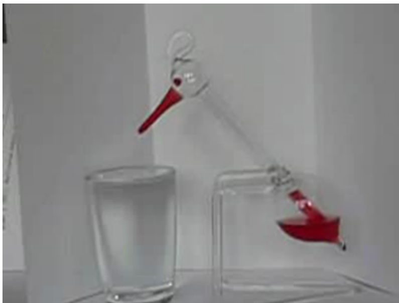
Figure 15.22 This novelty toy, known as the drinking bird, is an example of Carnot's engine. It contains methylene chloride (mixed with a dye) in the abdomen, which boils at a very low temperature—about 100^{\circ}\text{F} . To operate, one gets the bird's head wet. As the water evaporates, fluid moves up into the head, causing the bird to become top-heavy and dip forward back into the water. This cools down the methylene chloride in the head, and it moves back into the abdomen, causing the bird to become bottom heavy and tip up. Except for a very small input of energy—the original head-wetting—the bird becomes a perpetual motion machine of sorts. (credit: Arabesk.nl, Wikimedia Commons)
