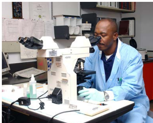
Figure 26.15 Multiple lenses and mirrors are used in this microscope. (credit: U.S. Navy photo by Tom Watanabe)
