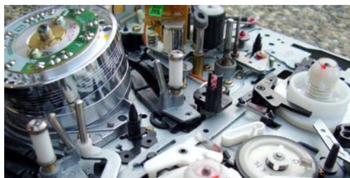
Figure 23.8 Recording and playback heads used with audio and video magnetic tapes. (credit: Steve Jurvetson)
