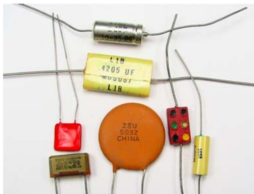
Figure 19.21 Some typical capacitors. Size and value of capacitance are not necessarily related. (credit: Windell Oskay)
