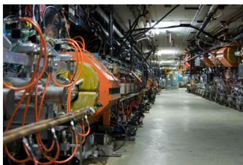
Figure 22.26 The Fermilab facility in Illinois has a large particle accelerator (the most powerful in the world until 2008) that employs magnetic fields (magnets seen here in orange) to contain and direct its beam. This and other accelerators have been in use for several decades and have allowed us to discover some of the laws underlying all matter. (credit: ammcgrim, Flickr)
