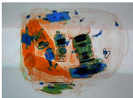
Figure 30.26 This x-ray image shows the contents of a piece of luggage. The denser the material, the darker the shadow. (credit: IDuke, Wikimedia Commons)
