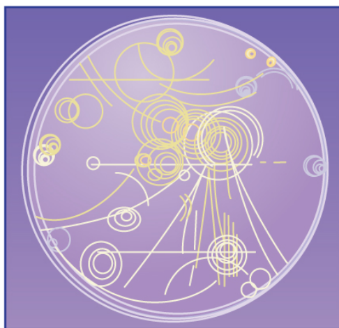
Figure 22.20 Trails of bubbles are produced by high-energy charged particles moving through the superheated liquid hydrogen in this artist's rendition of a bubble chamber. There is a strong magnetic field perpendicular to the page that causes the curved paths of the particles. The radius of the path can be used to find the mass, charge, and energy of the particle.
