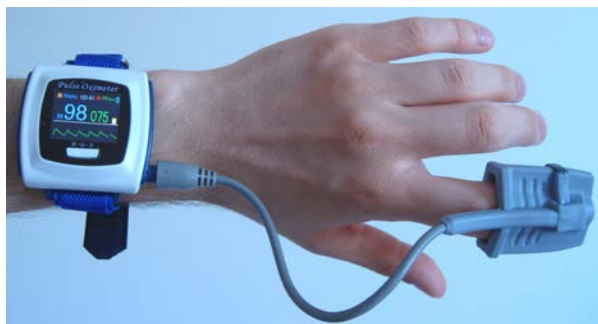
Figure 7.27 A pulse oximeter is an apparatus that measures the amount of oxygen in blood. Oxymeters can be used to determine a person's metabolic rate, which is the rate at which food energy is converted to another form. Such measurements can indicate the level of athletic conditioning as well as certain medical problems. (credit: UusiAjaja, Wikimedia Commons)
