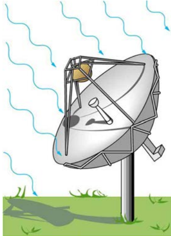
Figure 24.29 Satellite dishes receive TV signals sent from orbit. Although the signals are quite weak, the receiver can detect them by being tuned to resonate at their frequency.
